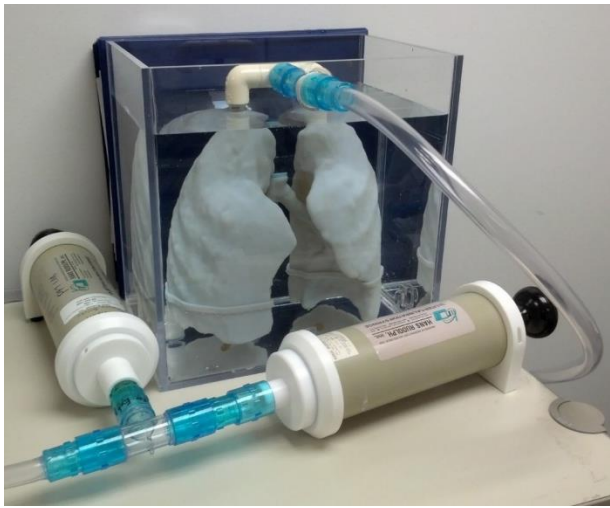
Figure 4. A lung phantom constructed by 3D printing based on the real lung shape derived from a static MRI image of a petite adult subject. Realistic tidal breathing effect by air volume and respiratory rate is simulated by pumping air into and out of the lung shell. See text for details.
