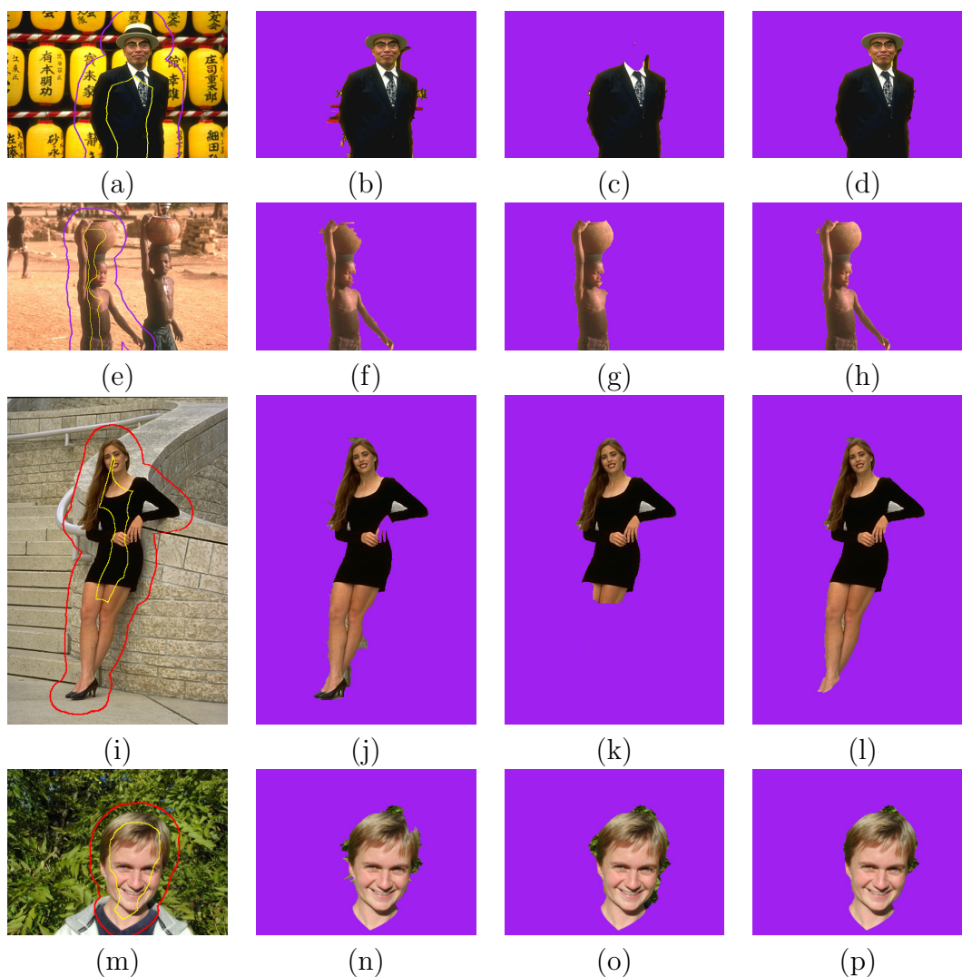
Figure 13: Results with seeds obtained by eroding and dilating the ground-truth. First column: Input images and seeds shown with solid colors. Second column: GC_{\max} results (more specifically IRFC, but PW outputs similar results). Third column: GC_{\text{sum}} results. Fourth column: GC_{\text{sum}}^{\max} results for the same seeds.
