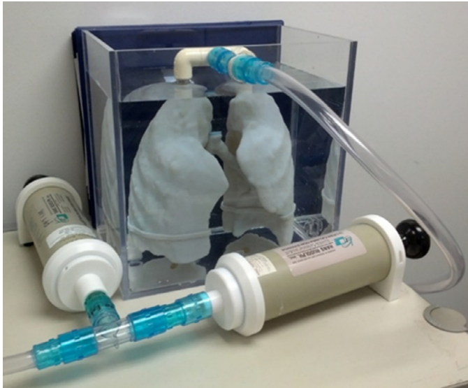
Fig. 4. A lung phantom constructed by 3D printing based on the real lung shape derived from a static MRI image of a petite adult subject. Realistic tidal breathing effect by air volume and respiratory rate is simulated by pumping air into and out of the lung shell. See text for details.
