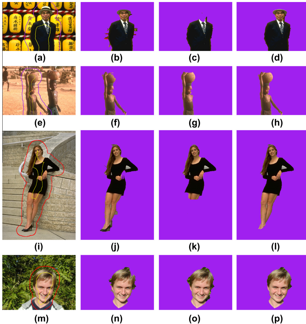
Fig. 13. Results with seeds obtained by eroding and dilating the ground-truth. First column: Input images and seeds shown with solid colors. Second column: GC_{max} results (more specifically IRFC, but PW outputs similar results). Third column: GC_{sum} results. Fourth column: GC_{sum}^{max} results for the same seeds.
